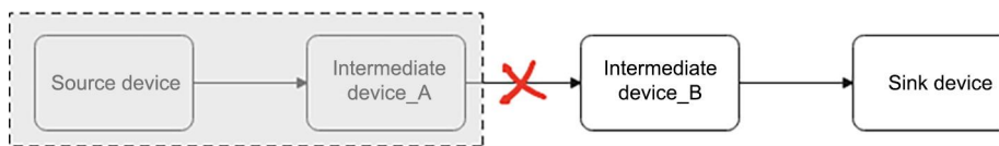
Figure 208 Schematic diagram of the scenario where an intermediate device port is unplugged
